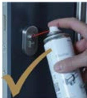
If using a thumbturn cylinder, it is recommended the door is opened using a cylinder pull and NOT the thumbturn on the cylinder as this will put unnecessary force on the cylinder and may cause it to snap.
