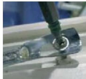
**Tighten screw to fix cord.**
