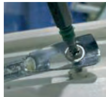
Tighten screw to fix cord. Clip shown may be different but fixing the same.
